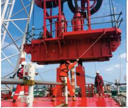
Fagioli operate a range of Jacks from 15 to 750 tonnes capacity each based upon lift cables of 1 to 50 strands of 18mm diameter, 7 wire die -compacted, prestressing strand of guaranteed minimum breaking load of 38 tonnes per strand.
